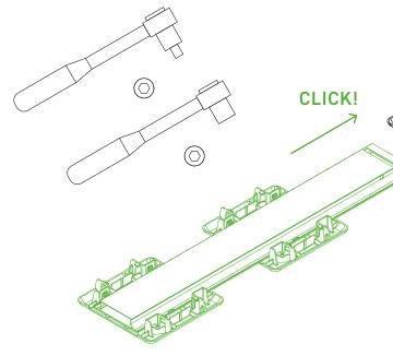
With the help of the track connection, cable tracks can be integrated along the system to ensure optimal cable management. In this case, the track bottom profile acts as an extension of the system in the rail direction in order to place the cable track there and screw it on. The track bottom profile must be pushed onto the base until the click detent engages with an audible noise. Fixing is done with a screw M8x16 through the hole in the profile into the base.
