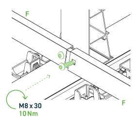
The cross strut connector  $\mathbf{G}$  must be installed at the specified locations according to the project report. This is to be pushed halfway into a transverse and ballast strut  $\mathbf{F}$ . The following transverse and ballast strut  $\mathbf{F}$  is to be pushed over the transverse strut connector. The component combination is attached to the tower  $\mathbf{D}$  with two M8 x 30 screws.
