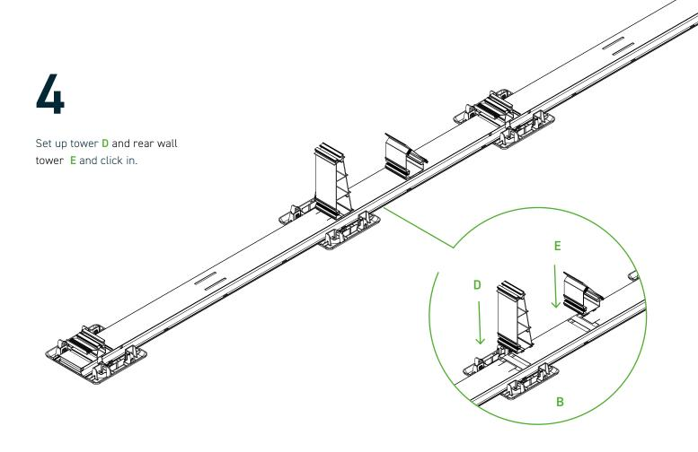
Press the tower  $\mathbf{D}$  with the detents pointing away from the centre of the rail and the rear wall tower  $\mathbf{E}$  with the detents pointing towards the centre of the rail vertically into the two narrow recesses of the main bottom profile  $\mathbf{B}$  and click the tower towards the rear wall tower and click the rear wall tower towards the base until the click detent clicks into place with audible noise.
