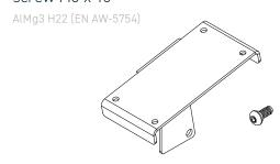
11 Mounting adapter for crossbar and ballast strut
