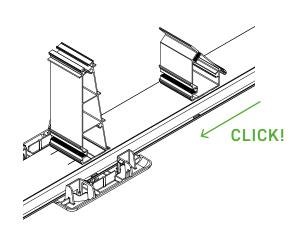
The detent connection must be checked for a clean fit and form fit (detent lug must be flush with the surface).
