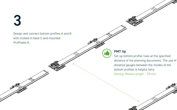
Lay out the main bottom profile  ${\bf B}$  with the base  ${\bf C}$  installed one after the other according to the project report.
