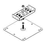
8 Track connection in module direction, screw 4.8 x 19
