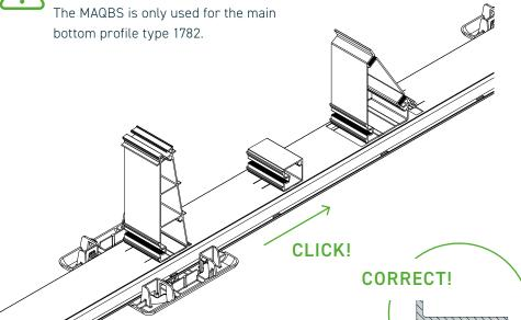
The detent connection must be checked for a clean fit and form fit (detent lug must be flush with the surface).
