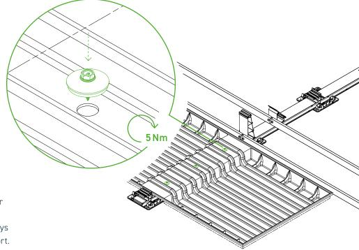
Place the ballast tray between the tower and base centrally on the main bottom profile. Exact positions of the ballast trays can be found in the current project report. Then screw each ballast tray centrally and evenly distributed on the main bottom profile by means of the supplied drilling screws (three pieces). Observe the maximum torque of 5 Nm!
