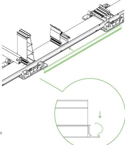
At the beginning, check the clean position and durable, secure fastening of the string lines to avoid damage to the lines due to movements (wind).
