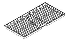
Remove gravel/substrate fill up to the inner edges of the main bottom profiles in the area between base and tower. The depth of the excavation should be at least 50 mm from the top edge of the bed, in order to ensure that the ballast tray rests flat on the remaining bed or the roof surface. When placing the ballast tray directly on the roof covering, care must be taken to ensure a clean surface in order to avoid long-term damage.
