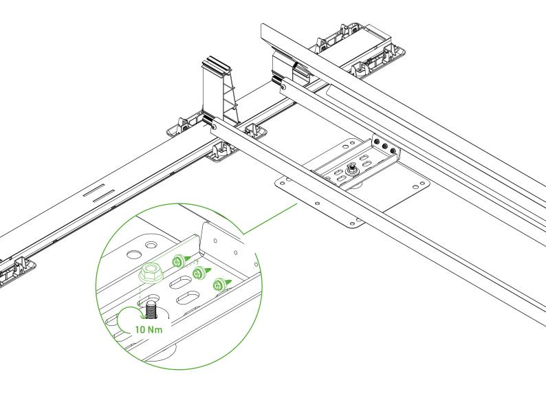
To attach the connection point to the system, three supplied drilling screws are screwed into the transverse and ballast struts on each side through the USO sheet. The location and position of the USO connection can be found in the current project documents.
