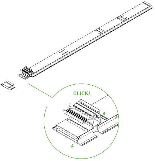
The base  ${\bf C}$  is to be pushed into the main bottom profile  ${\bf B}$  until the click lock engages with an audible noise. One base must be installed per main bottom profile. At the beginning and end of a main bottom strand, a starting and end bottom profile  ${\bf A}$  must also be clicked onto the base  ${\bf C}$ .
