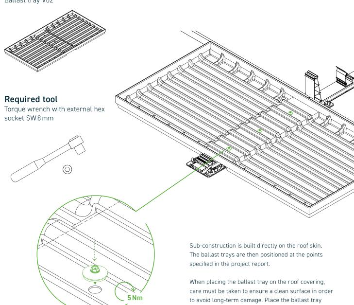
between the tower and base centrally on the main bottom profile. Exact positions of the ballast trays can be found in the current project report. Then screw each ballast tray centrally and evenly distributed on the main bottom profile by means of the supplied
