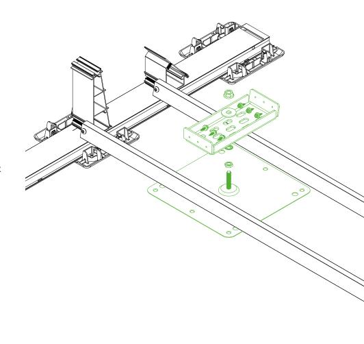
The fastening points of the USO connection should be mounted/installed on the roof before mounting the system. The attachment point should be positioned as centrally as possible between the surrounding tower or rear wall tower in the vicinity of a main bottom profile. A nut of flat design (DIN-EN-ISO 4035) and a fan washer are screwed onto the threaded bolt of the fastening point. The fan washer later serves as a support for the uso sheet metal.
