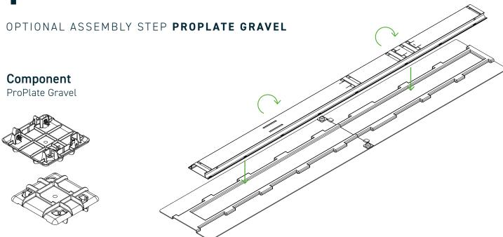
Turn the main floor profile over and place it upside down in the ClickGuide ReUse. Then position the ProPlates Gravel and snap in place. The exact placement of the ProPlates Gravel can be found in the data sheet with the corresponding assignment variants.
