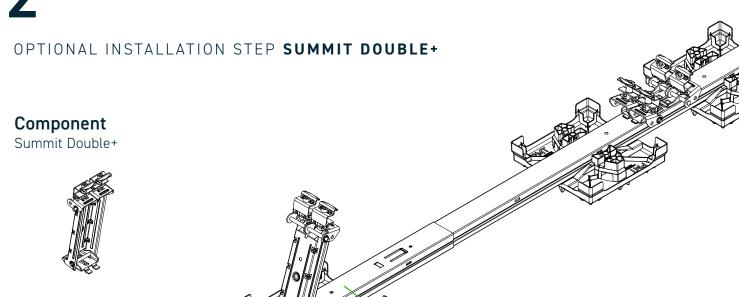
Press the Summit Double+ with the locking lugs vertically into the recesses of the Swift Rail Short and push it towards the middle of the rail until you hear a click.
