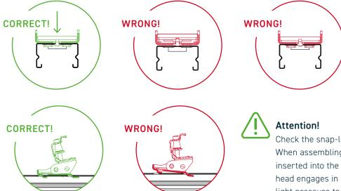
Check the snap-lock joint to ensure it fits perfectly. When assembling, ensure that all 4 locking tabs are inserted into the recess provided and that the hammer head engages in the corresponding T-recess. Apply light pressure to the hammer head to ensure that it assumes its final position.
