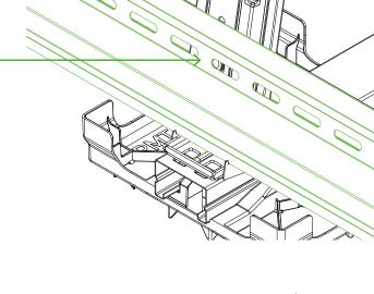
Place Swift Shield or Swift Shield Link on the back of the Summit Single+ and slide it down into the cut-out provided.
