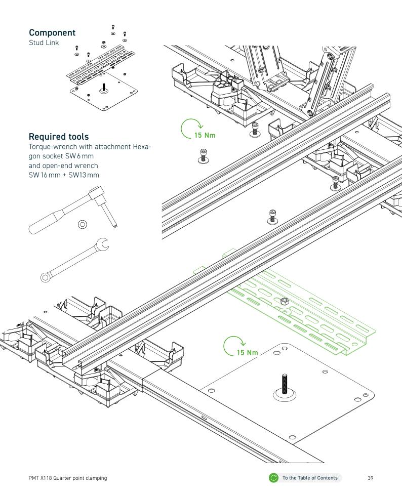
The Stud Link attachment points are located on the Row Connector or Row Link and should be fitted before the Stud Link is assembled. The Stud Link connection should be fixed as close as possible to a rail.
