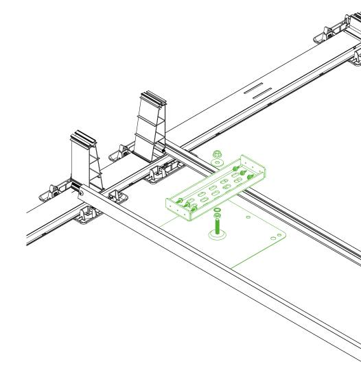
The fastening points of the USO connection should be positioned near a main bottom profile before mounting the system on the roof. The attachment point should be positioned as centrally as possible between the four surrounding towers. A nut of flat design (DIN-EN-ISO 4035) and a fan washer are screwed onto the threaded bolt of the fastening point. The fan washer later serves as a support for the uso sheet metal.
