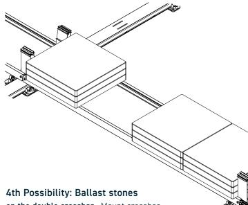
on the double crossbar. Mount crossbar and ballast strut on both sides of the tower as described in step 5, place ballast stones evenly distributed on the crossbars near the tractor.
