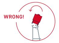
Attach the mid and end clamps  ${\bf I}$  on the side of the tower  ${\bf E}$  facing the base **C** to the lower guide groove and press them onto the opposite guide groove until the click lock engages with an audible noise.
