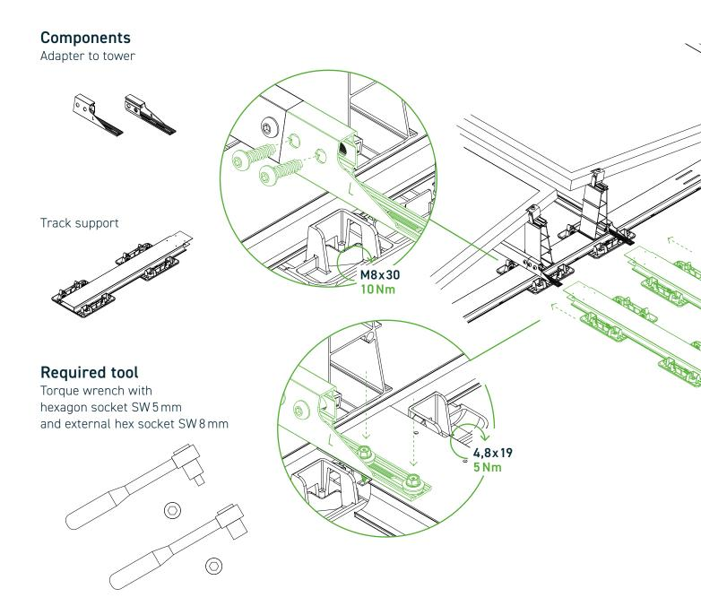
First, the support of the track is defined by the recess on the underside of the profile, since there the web of the ProPlat is inserted.
