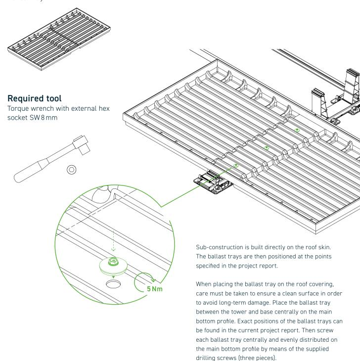
Subsequently, the bed is distributed smoothly in the ballast trays and on the bottom profiles.
