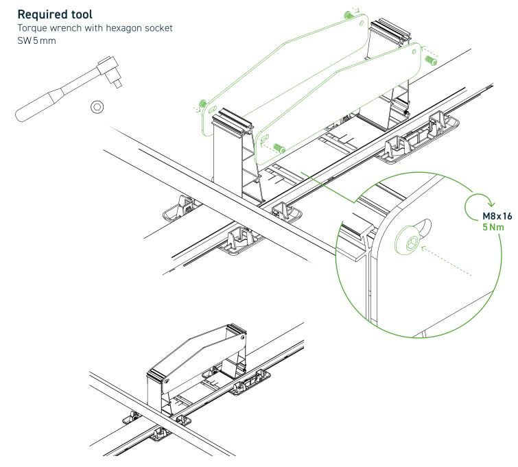
OPTIONAL ASSEMBLY STEP IRRADIATION SENSOR BRACKET
