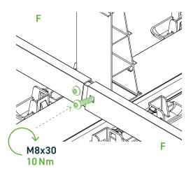
The cross strut connector  $\mathbf{G}$  must be installed at the specified locations according to the project report. This is to be pushed halfway into a transverse and ballast strut  $\mathbf{F}$ . The following transverse and ballast strut  $\mathbf{F}$  is to be pushed over the transverse strut connector. The component combination is attached to the tower  $\mathbf{E}$  with two screws M8 x 30.
