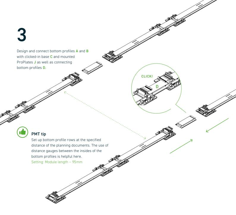
Lay out the main bottom profile  ${\bf B}$  with the base  ${\bf C}$  installed one after the other according to the project report.
