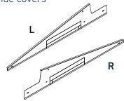
First remove the pre-punched recesses for the ballast stones in the side covers according to the information from the current project report. These are cut with the help of a side cutter and separated by bending.
