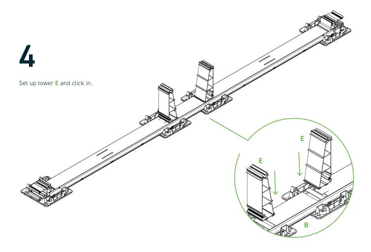
Press the two central components tower  $\mathbf{E}$  with the detents pointing towards the centre of the rail, vertically into the two narrow recesses of the main bottom profile  $\mathbf{B}$  and push them towards the centre of the rail until the click detent clicks into place with an audible noise.
