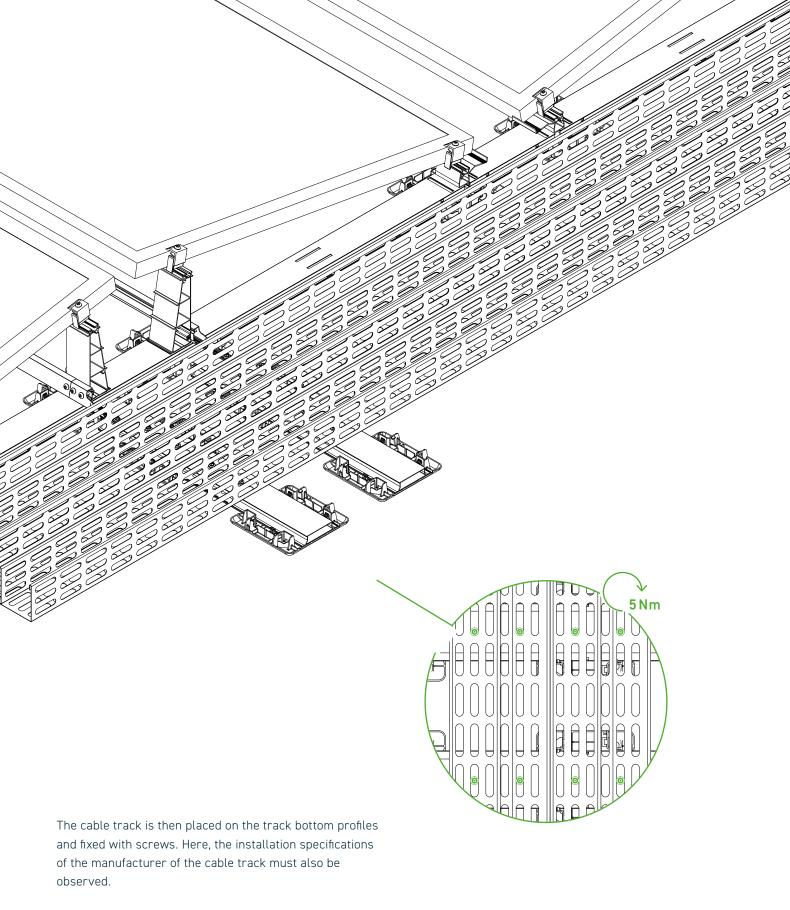
The exact location and position of the adapters on the tower, the track bottom profiles and the cable tracks can be found in the current project documents.
