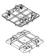
Turn the main floor profile over and place it upside down in the ClickGuide ReUse. Then position the ProPlates Gravel and snap in place. The exact placement of the ProPlates Gravel can be found in the data sheet with the corresponding assignment variants.
