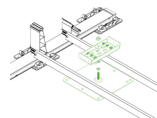
The fastening points of the USO connection should be mounted/installed on the roof before mounting the system. The attachment point should be positioned as centrally as possible between the surrounding tower or rear wall tower in the vicinity of a main bottom profile. A nut of flat design (DIN-EN-ISO 4035) and a fan washer are screwed onto the threaded bolt of the fastening point. The fan washer later serves as a support for the uso sheet metal.
