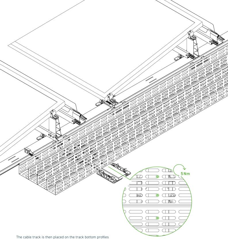
and fixed with screws. Here, the installation specifications of the manufacturer of the cable track must also be observed.
