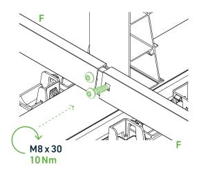
The cross strut connector **G** must be installed at the specified locations according to the project report. This is to be pushed halfway into a transverse and ballast strut **F**. The following transverse and ballast strut **F** is to be pushed over the transverse strut connector. The component combination is attached to the tower **D** with two M8 x 30 screws.
