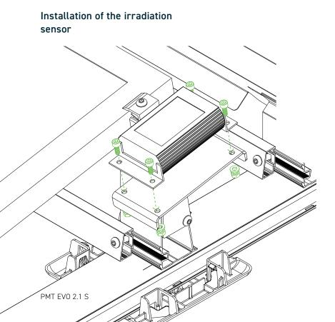
Using the bracket for the irradiation sensor it can be easily integrated into the system. The carrier plate is mounted on the tower with two screws. The exact location and position of the bracket can be found in the current project documents.
