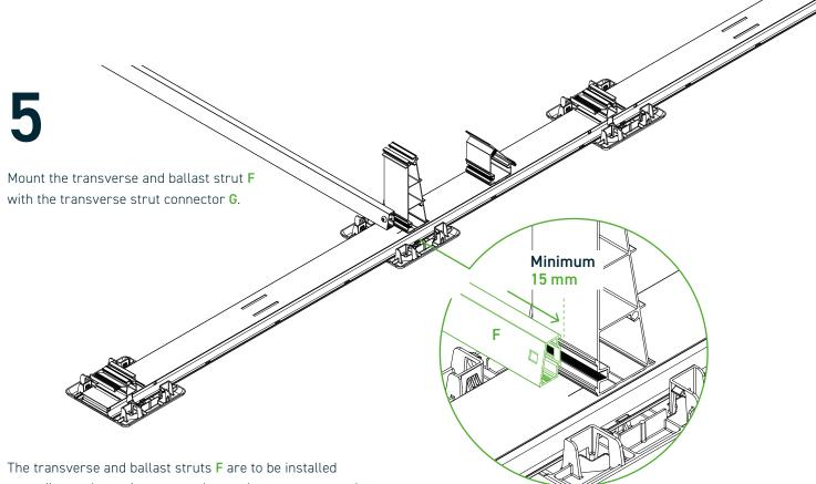
The transverse and ballast struts **F** are to be installed according to the project report. Insert the transverse and ballast strut **F** centrally between the components tower **E** into the mounting lugs.
