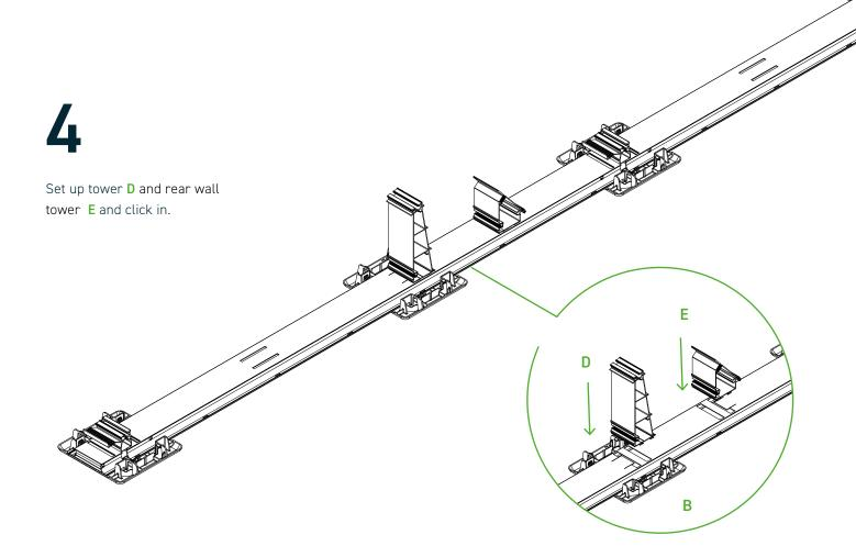
Press the tower **D** with the detents pointing away from the centre of the rail and the rear wall tower **E** with the detents pointing towards the centre of the rail vertically into the two narrow recesses of the main bottom profile **B** and click the tower towards the rear wall tower and click the rear wall tower towards the base until the click detent clicks into place with audible noise.
