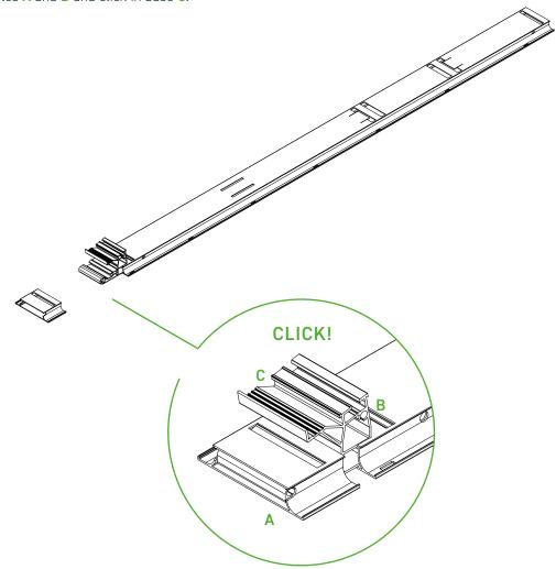
The base **C** is to be pushed into the main bottom profile **B** until the click lock engages with an audible noise. One base must be installed per main bottom profile. At the beginning and end of a main bottom strand, a starting and end bottom profile **A** must also be clicked onto the base **C**.
