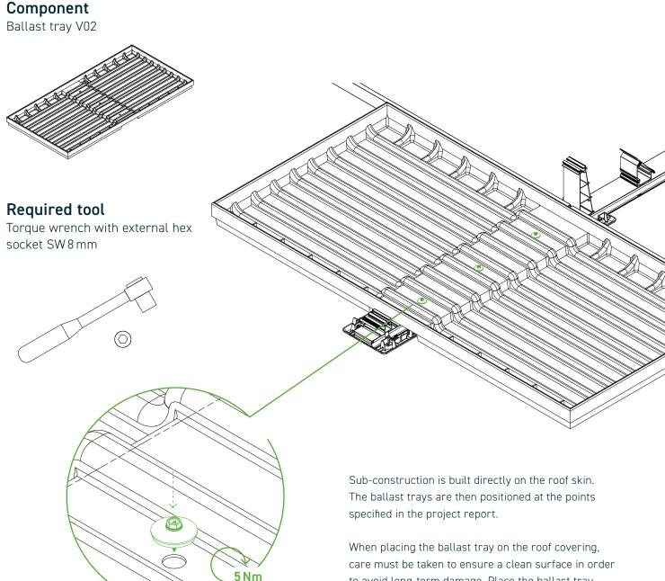
care must be taken to ensure a clean surface in order to avoid long-term damage. Place the ballast tray between the tower and base centrally on the main bottom profile. Exact positions of the ballast trays can be found in the current project report. Then screw each ballast tray centrally and evenly distributed on the main bottom profile by means of the supplied drilling screws (three pieces).
