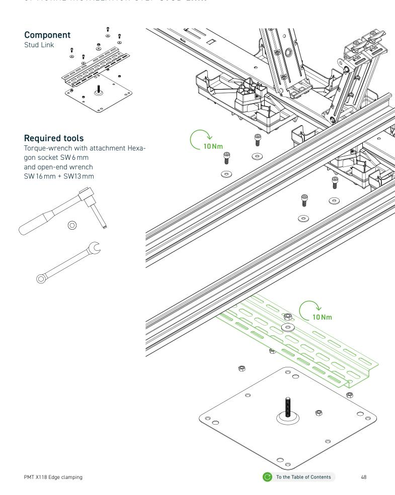
The Stud Link attachment points are located on the Row Connector Edge or Row Link Edge and should be fitted before the Stud Link is assembled. The Stud Link connection should be fixed as close as possible to a rail.
