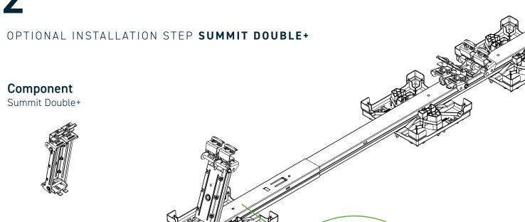
Press the Summit Double+ with the locking lugs vertically into the recesses of the Swift Rail Short and push it towards the middle of the rail until you hear a click.
