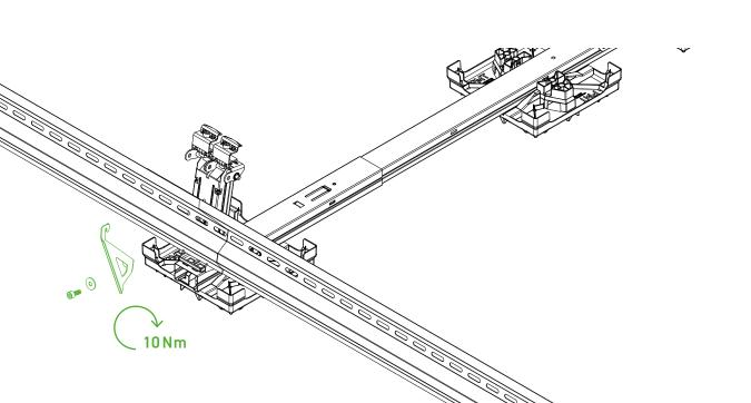
Place the Swift Shield Bracket in the position of a Summit Double+ on Swift Shield Link and Swift Shield.
