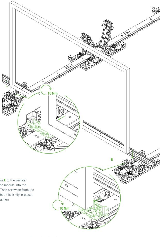
Move the Pivot Double  ${\bf E}$  to the vertical position and insert the module into the clamps from above. Then screw on from the rear side, checking that it is firmly in place and in the correct position.
