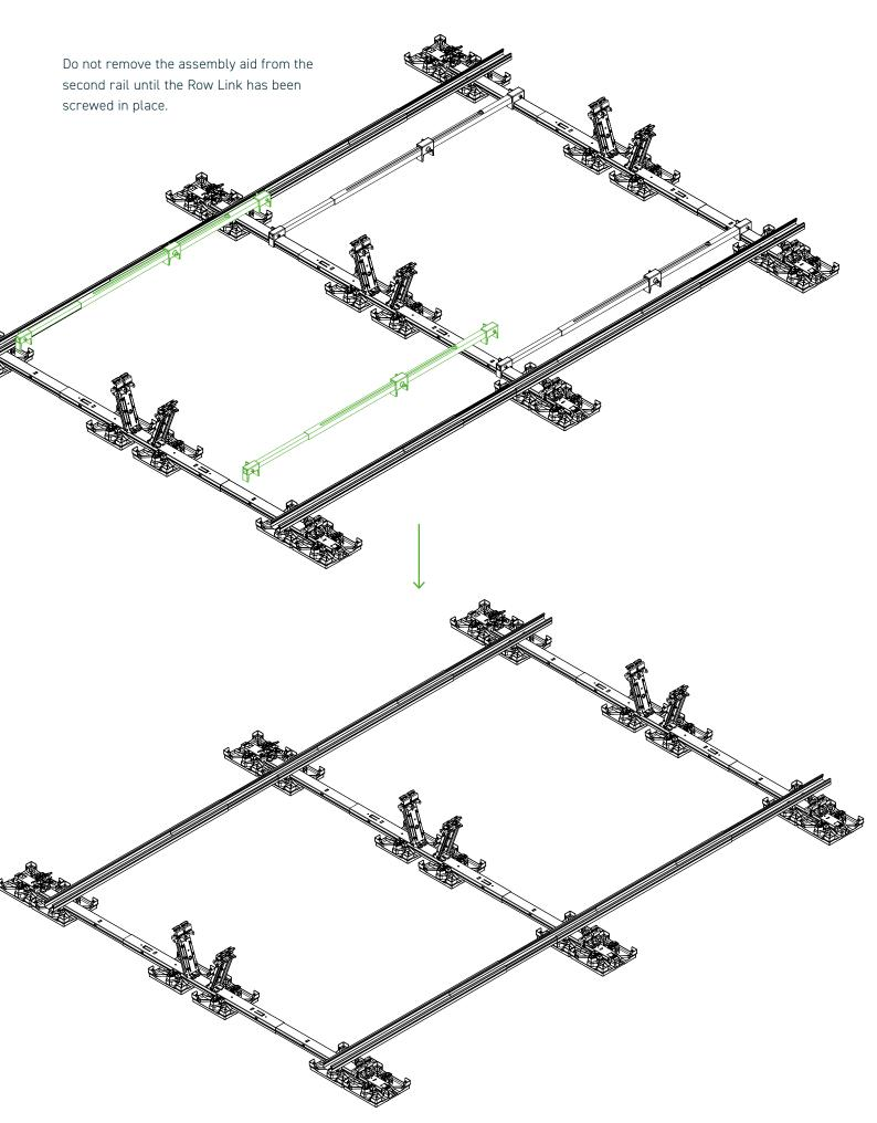
4.7 Use of the assembly aid at the end of the module field. Align the mounted and positioned rails using the previously set assembly aid. Module field edge-END
