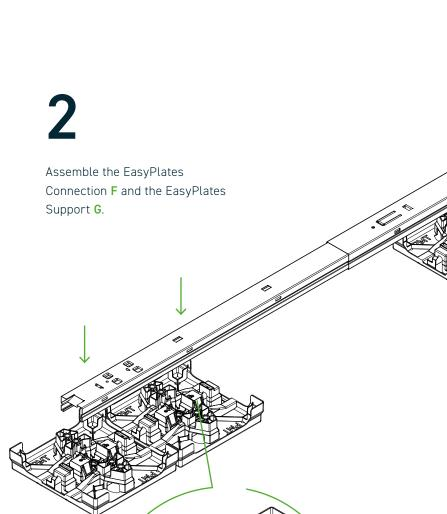
Place the already snapped in Swift Rail Short B with Swift Rail Connector C and Swift Rail A on the EasyPlates and snap them in the cut-outs provided. The EasyPlates can also be installed at the same time individual Swift components are assembled.
