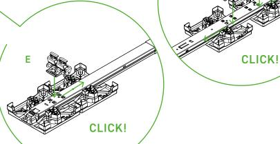
Press the Pivot Double **E** with the locking lugs vertically into the recesses of the Swift Rail Short **B** and push it towards the middle of the rail until you hear a click. With Swift Rail **A**, the Pivot Double **E** must be placed with the locking lugs pointing away from the centre of the rail and locked in place.
