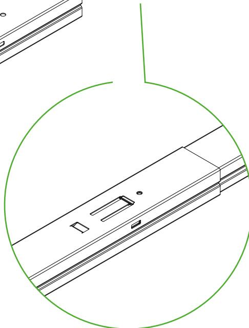
Slide the Swift Edge into the Swift Connector profile until you hear a click. At the beginning and end of a complete string, a Swift Edge must be pushed onto the Swift Connector.
