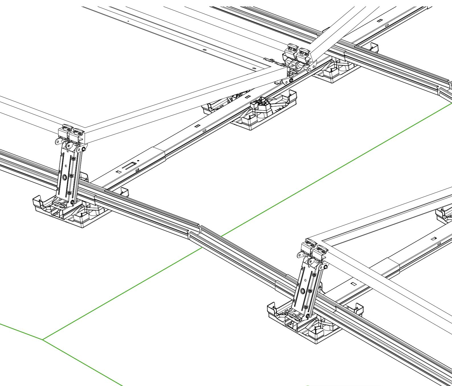
First, the ridge line is determined. Then the Swift Rail profiles are assembled (parallel to the ridge).
