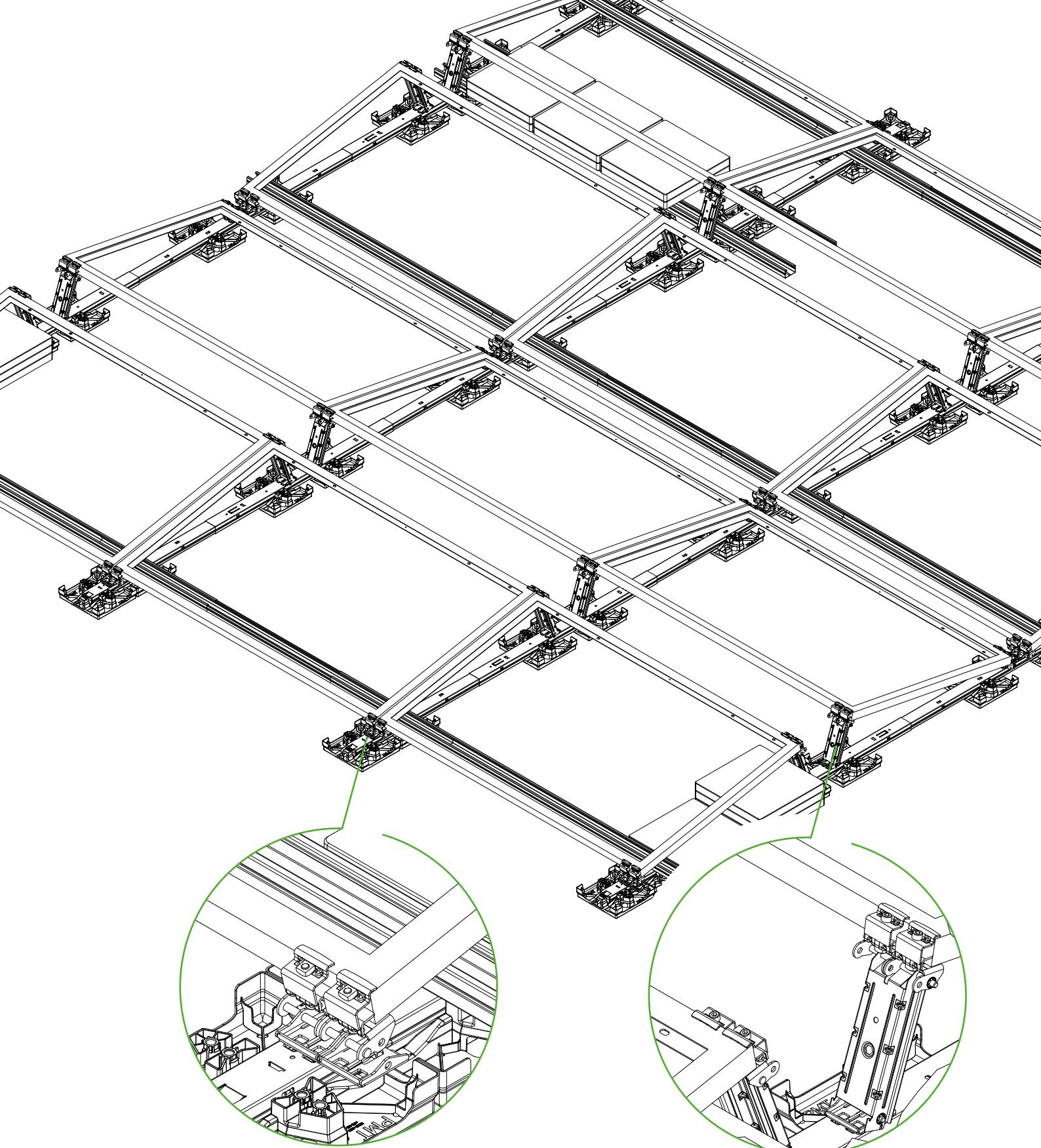
At the end of a system, the Pivot Double and Summit Double can be mounted with both clamps over the module frame.
