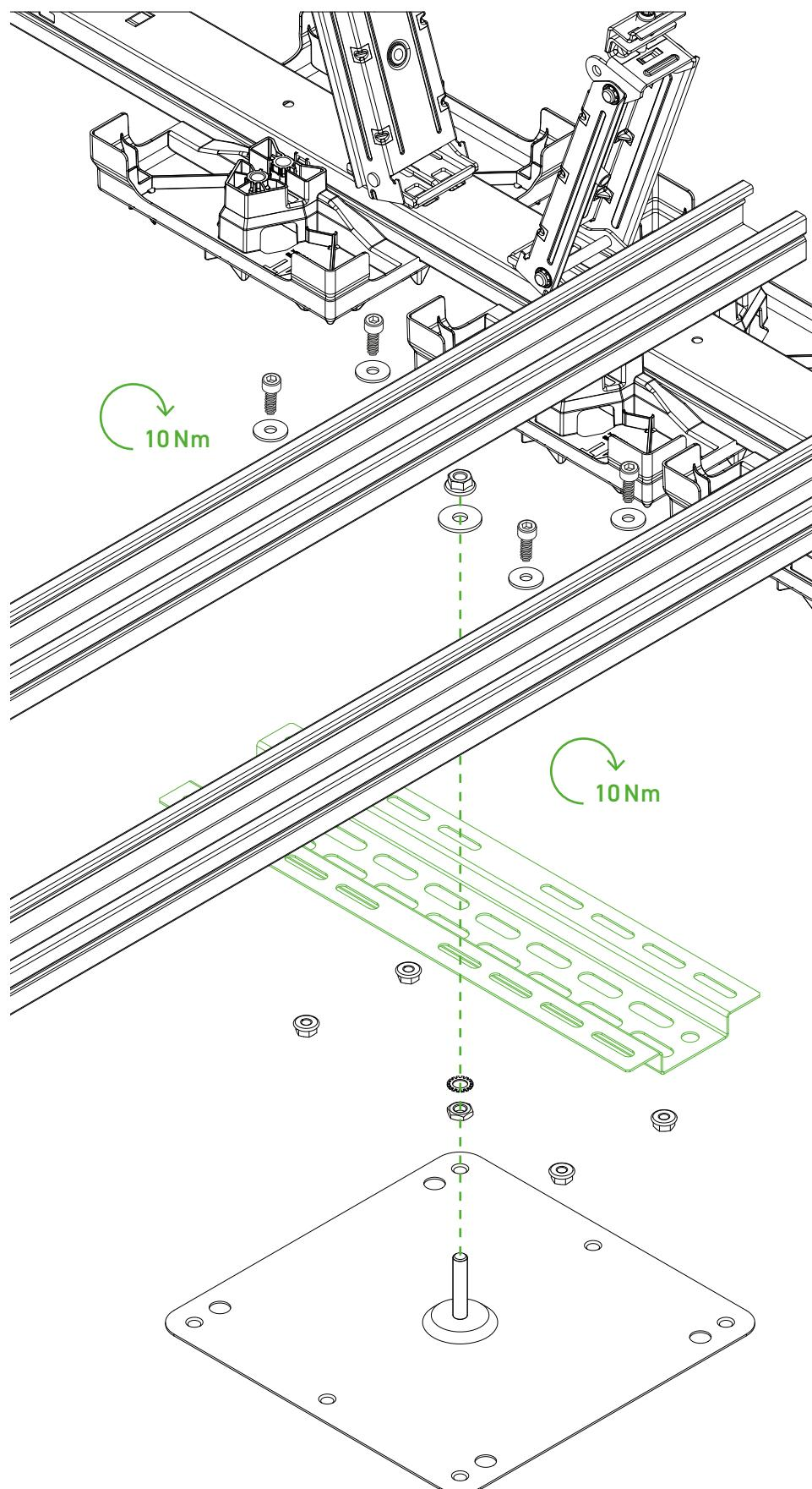
The Stud Link attachment points are located on the Row Connector Edge or Row Link Edge and should be fitted before the Stud Link is assembled. The Stud Link connection must be fastened at a distance of at least 150 mm and no more than 400 mm from the rail.
