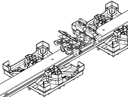
Press the Summit Double+ with the locking lugs vertically into the recesses of the Swift Rail Short and push it towards the middle of the rail until you hear a click.
