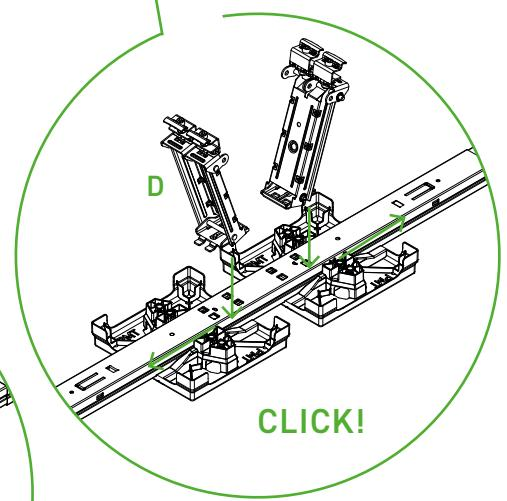
Press the Pivot Double **E** with the locking lugs vertically into the recesses of the Swift Rail Short **B** and push it towards the middle of the rail until you hear a click. With Swift Rail **A**, the Pivot Double **E** must be placed with the locking lugs pointing away from the centre of the rail and locked in place.
