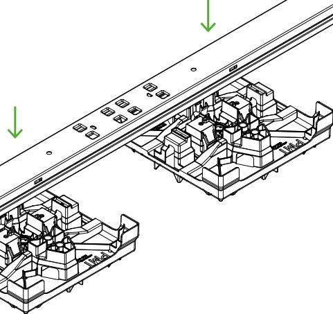
Place the already snapped in Swift Rail Short with Swift Rail Connector and Swift Rail on the EasyPlates Gravel and snap them in the cut-outs provided. The EasyPlates Gravel can also be installed at the same time individual Swift components are assembled.
