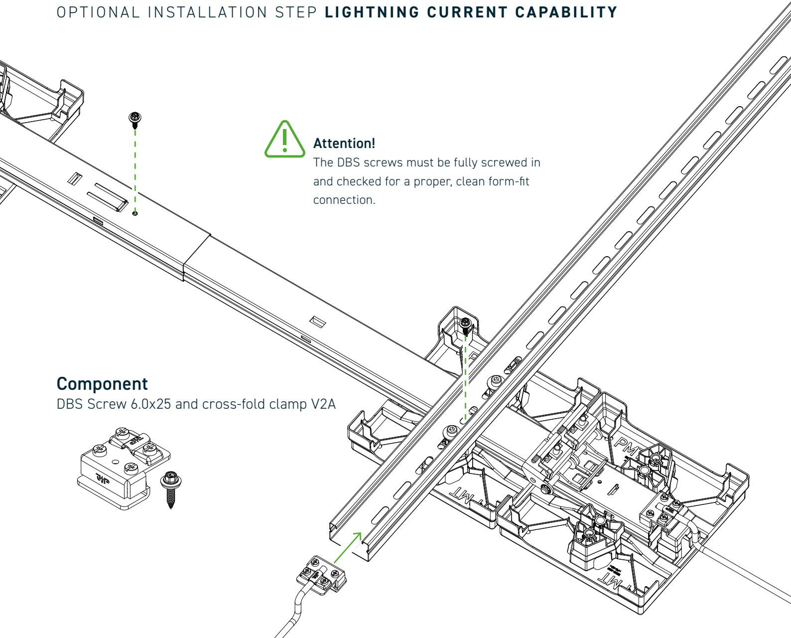
Our PMT X118 system (lower grid with corresponding measures) is capable of carrying lightning currents. This does not automatically mean that the building's external lightning protection can be integrated in accordance with lightning protection class 3 (PV system > 100 kWp).
