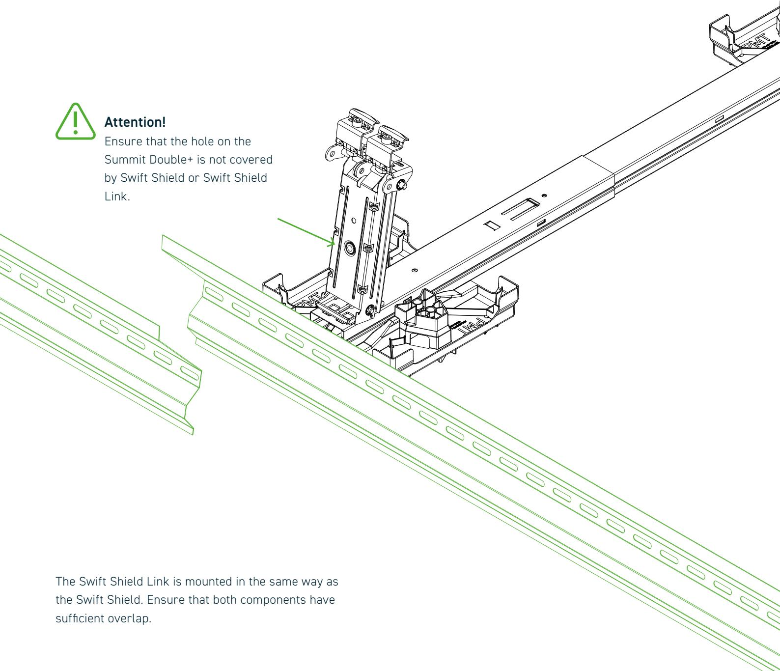
The Swift Shield Link is mounted in the same way as the Swift Shield. Ensure that both components have sufficient overlap.
