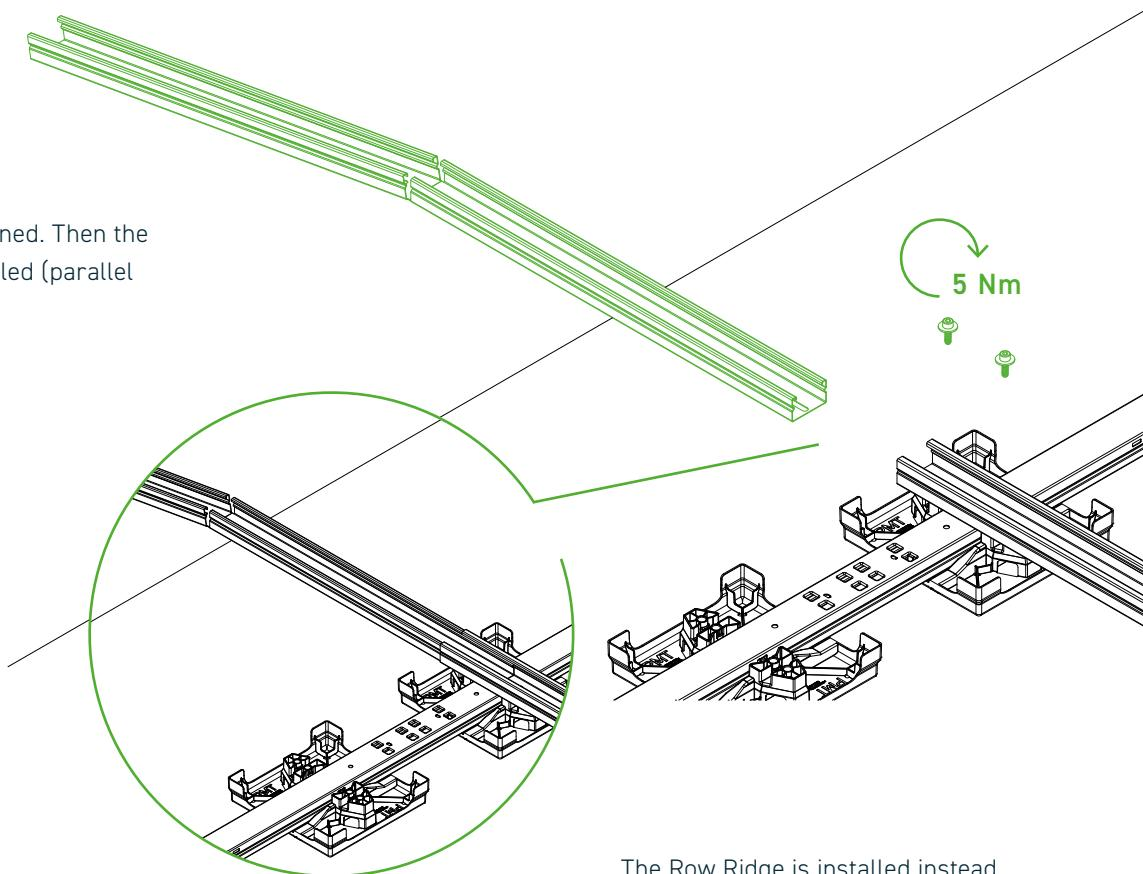
The Row Ridge is installed instead of a Row Link. The structure should be assembled evenly on both sides to prevent lopsided loading and thus slipping. Always refer to the current project documents for the location and position of the ridge connectors.
