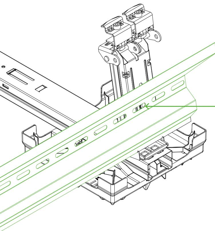
Place Swift Shield or Swift Shield Link on the back of the Summit Double+ and slide it down into the cut-out provided.
