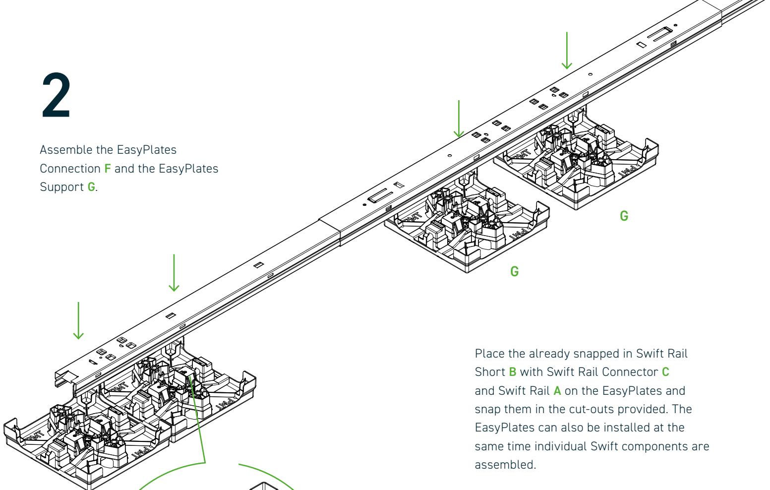
Place the already snapped in Swift Rail Short **B** with Swift Rail Connector **C** and Swift Rail **A** on the EasyPlates and snap them in the cut-outs provided. The EasyPlates can also be installed at the same time individual Swift components are assembled.
