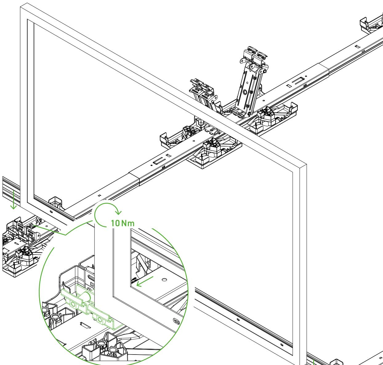
Move the Pivot Double **E** to the vertical position and insert the module into the clamps from above. Then screw on from the rear side, checking that it is firmly in place and in the correct position.
