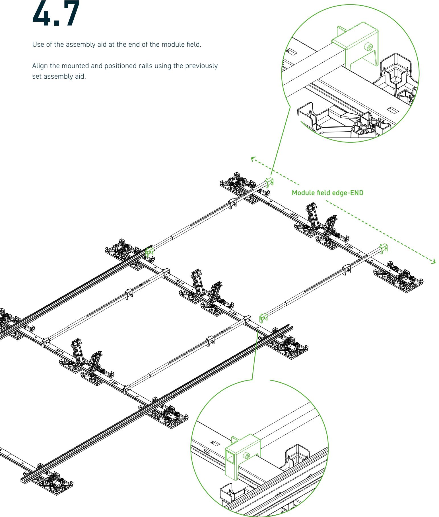
Slide Row Link Edge into Row Connector Edge, place on EasyPlate Connection and mount.
