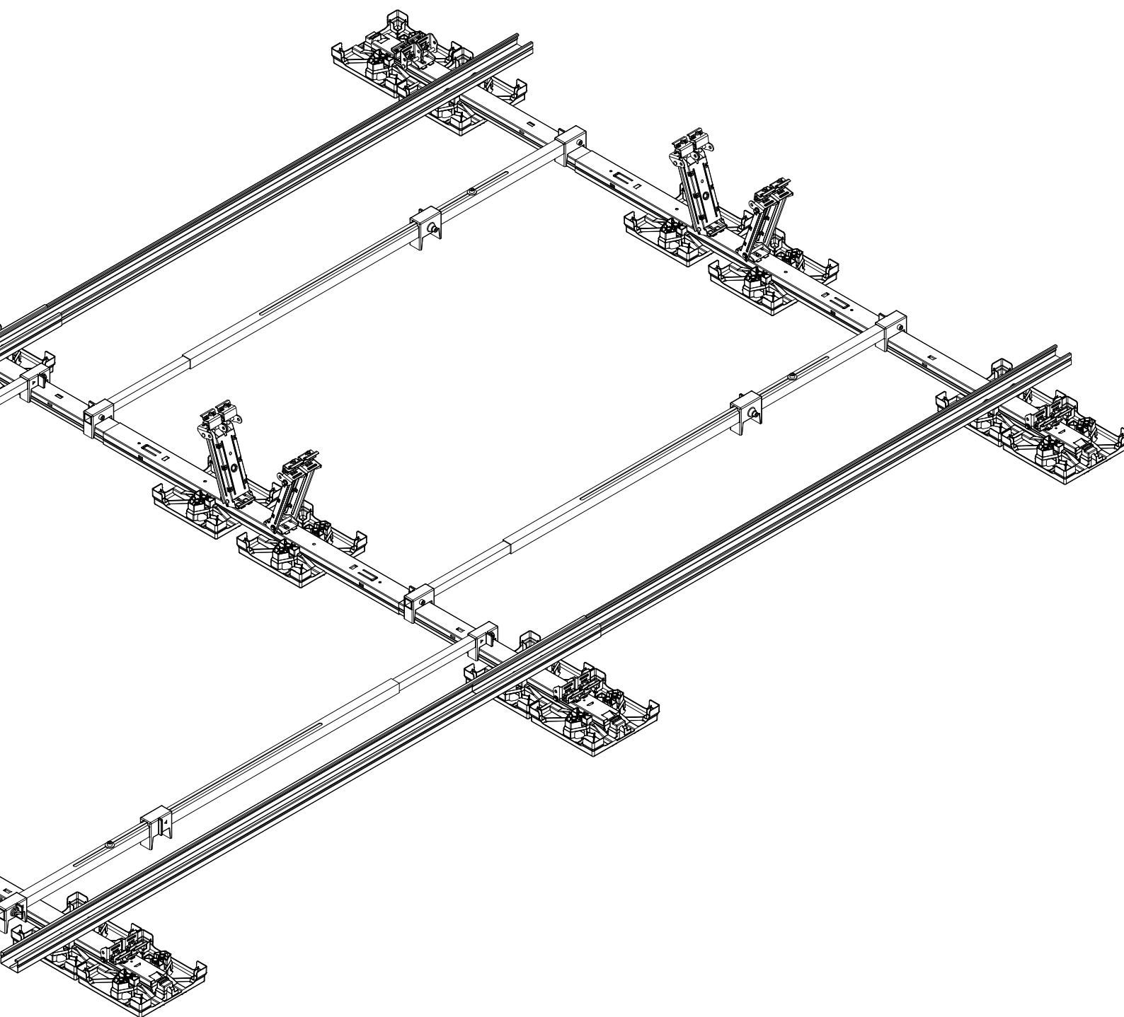
Do not remove the assembly aid from the second rail until the Row Link has been screwed in place.
