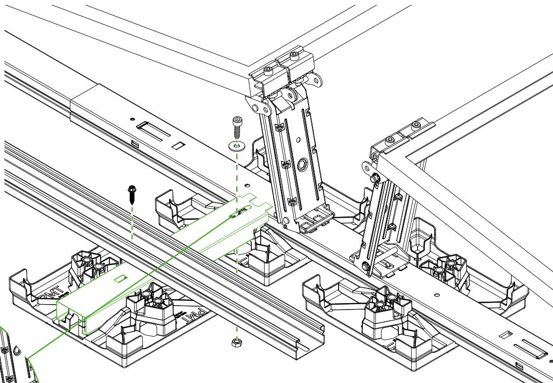
The Route Connection is first clicked into the Easy Plate Support. It is then fastened laterally to the system using an M8x25 hex socket screw, a washer, and a hex nut, and tightened to 5 Nm.
