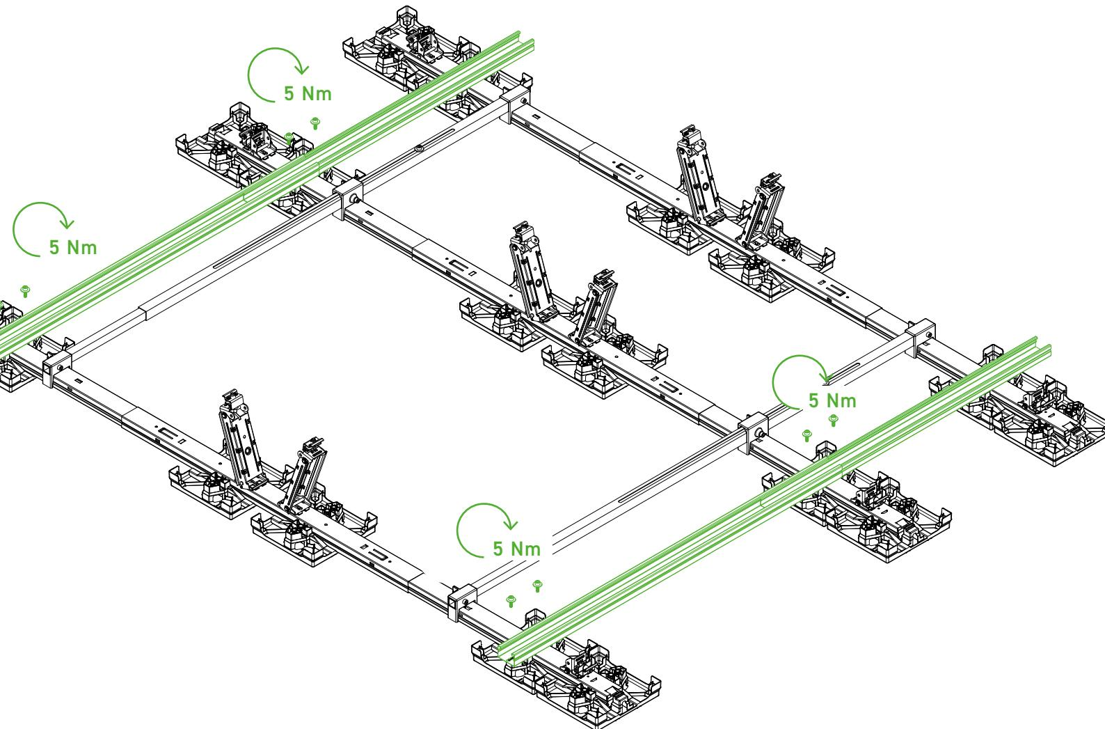
Row Connector **I**, Row Link **J** and EasyPlate Connection **F** must be mounted at the specified locations in accordance with the project report.
