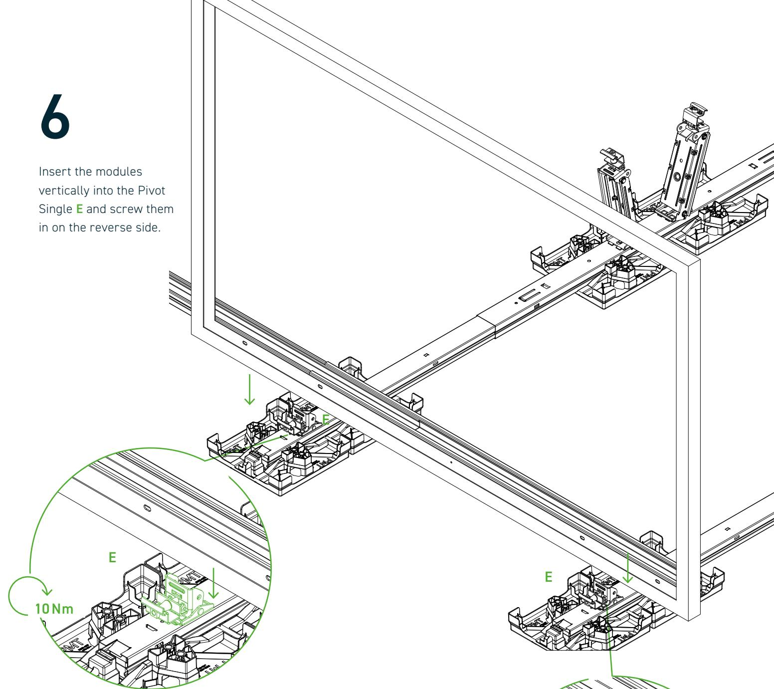
Place the Pivot Single **E** in a vertical position and insert the module into the clamps from above. Then screw on from the rear side, checking that it is firmly in place and in the correct position.
