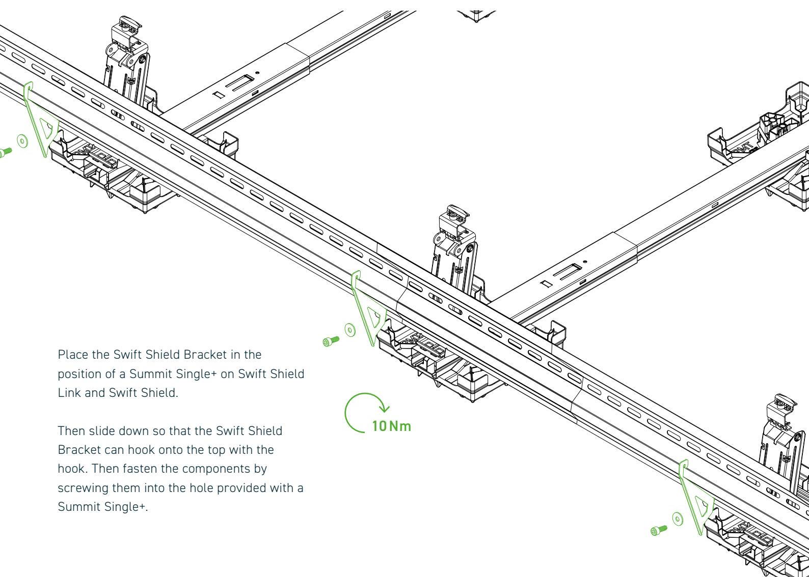
Place the Swift Shield Bracket in the position of a Summit Single+ on Swift Shield Link and Swift Shield.
