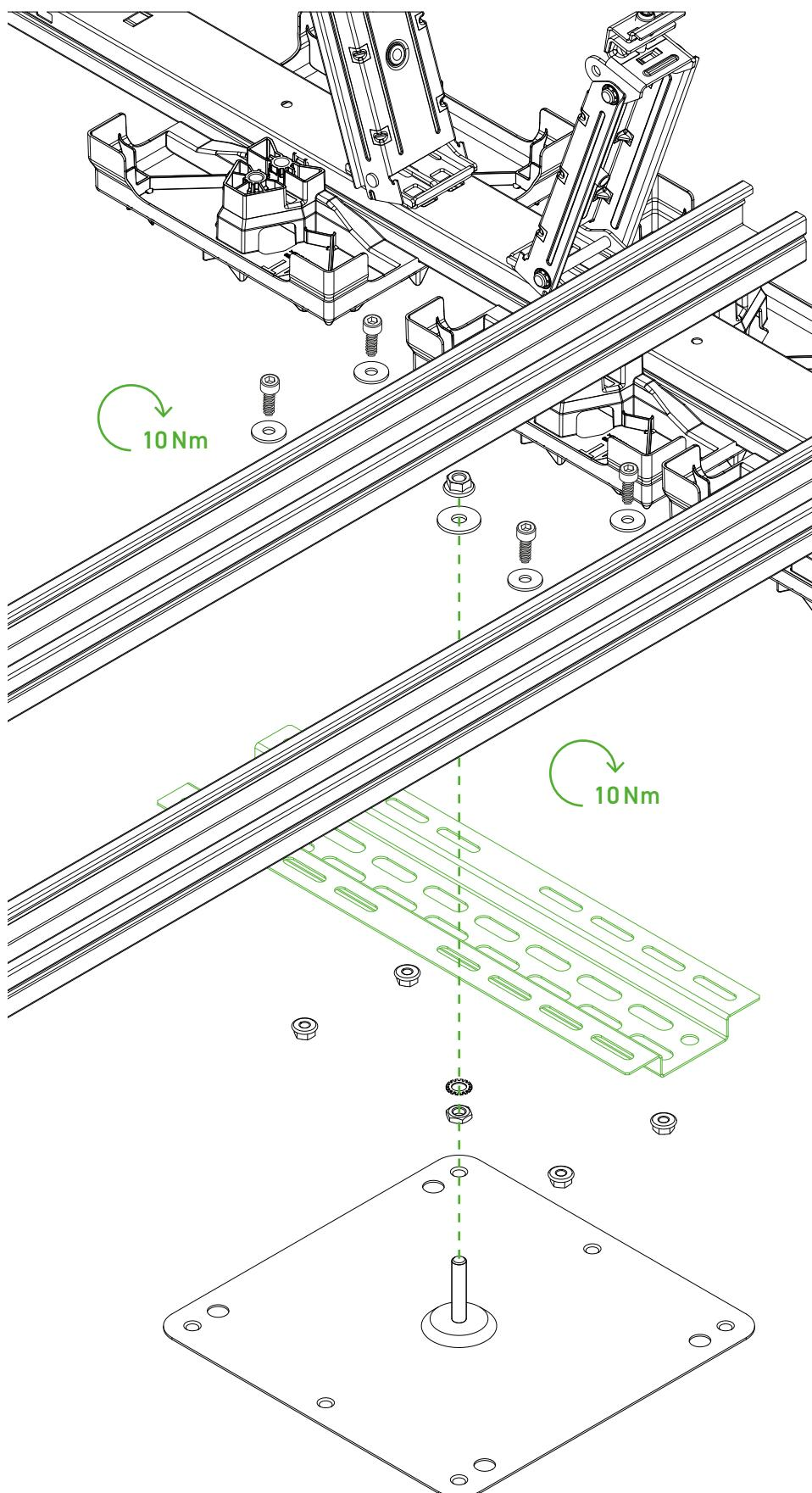
The Stud Link attachment points are located on the Row Connector or Row Link and should be fitted before the Stud Link is assembled. The Stud Link connection must be fastened at a distance of at least 150 mm and no more than 400 mm from the rail.
