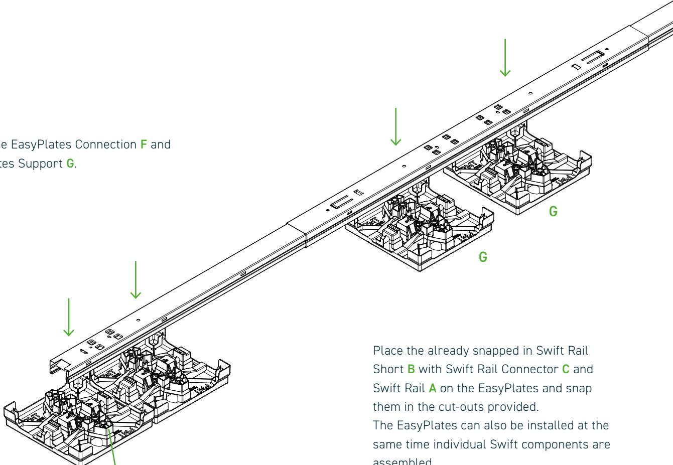
Place the already snapped in Swift Rail Short **B** with Swift Rail Connector **C** and Swift Rail **A** on the EasyPlates and snap them in the cut-outs provided.
