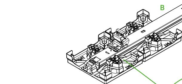
Press the Pivot Single **E** with the locking lugs vertically into the recesses of the Swift Rail Short **B** and push it towards the middle of the rail until you hear a click. With Swift Rail **A**, the Pivot Single **E** must be placed with the locking lugs pointing away from the centre of the rail and locked in place.
