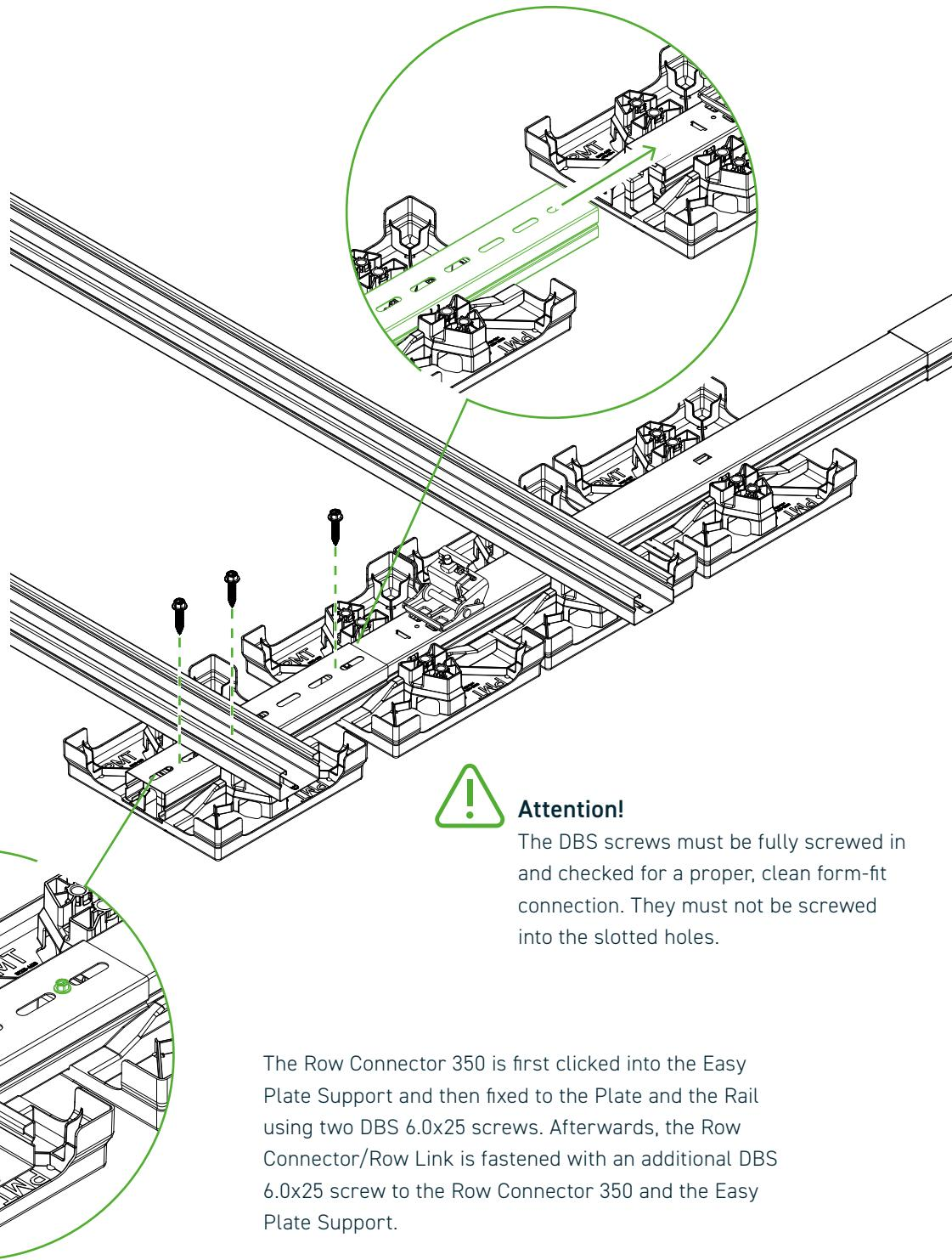
The Row Connector 350 is first clicked into the Easy Plate Support and then fixed to the Plate and the Rail using two DBS 6.0x25 screws. Afterwards, the Row Connector/Row Link is fastened with an additional DBS 6.0x25 screw to the Row Connector 350 and the Easy Plate Support.
