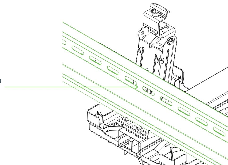
Place Swift Shield or Swift Shield Link on the back of the Summit Single+ and slide it down into the cut-out provided.
