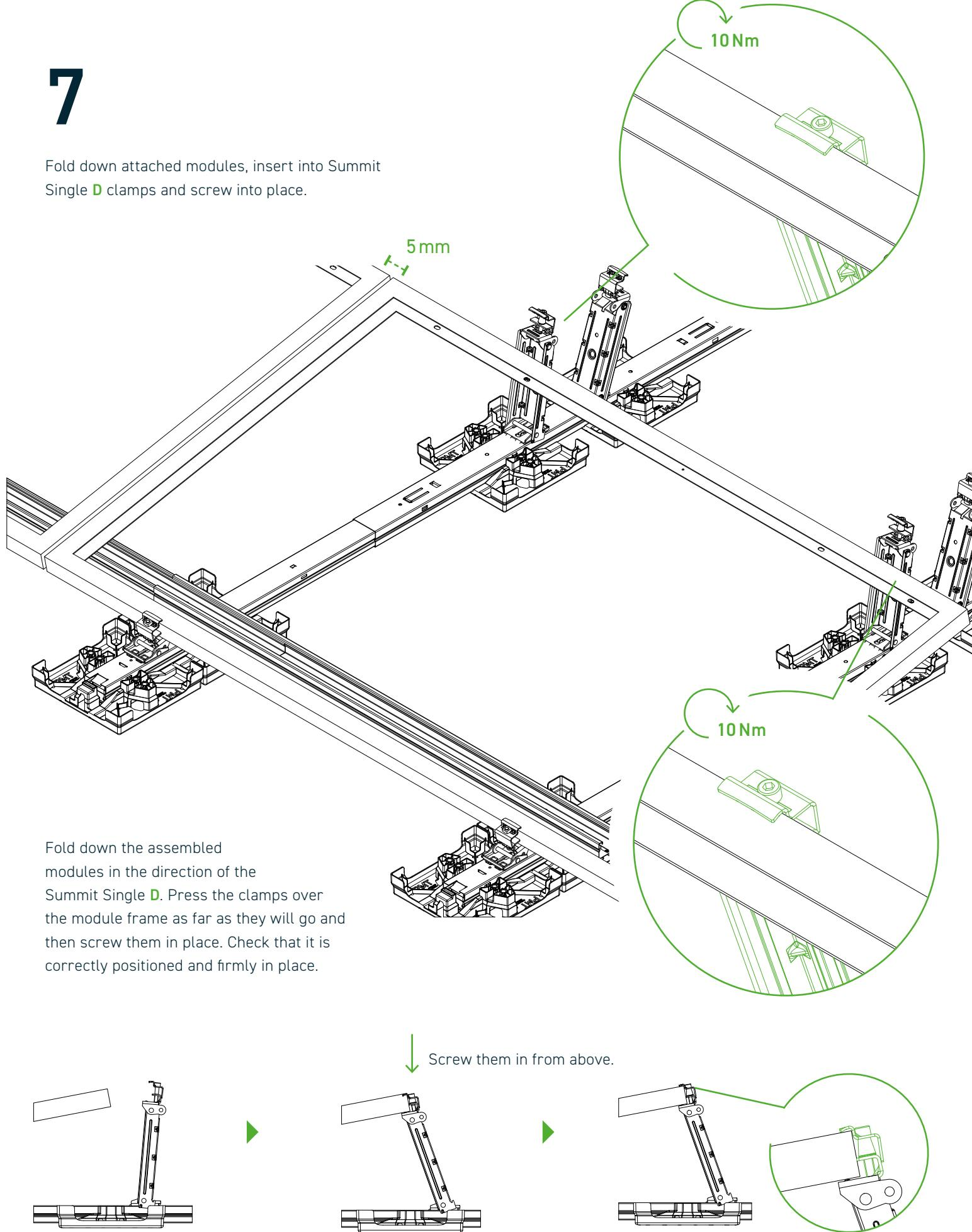
Fold down the assembled modules in the direction of the Summit Single **D**. Press the clamps over the module frame as far as they will go and then screw them in place. Check that it is correctly positioned and firmly in place.
