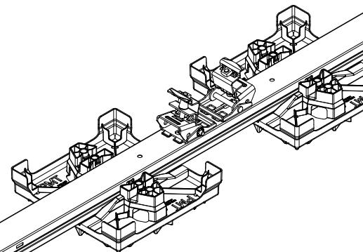
Press the Summit Single+ with the locking lugs vertically into the recesses of the Swift Rail Short and push it towards the middle of the rail until you hear a click.
