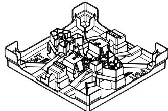
Cable trays can be fastened to the Easy Plates Support using two DBS 6.0x25 screws each.
