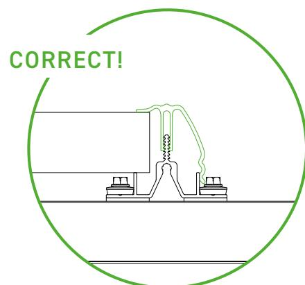
The end clamps must be placed at an angle to the rail screw due to the risk of tilting.
