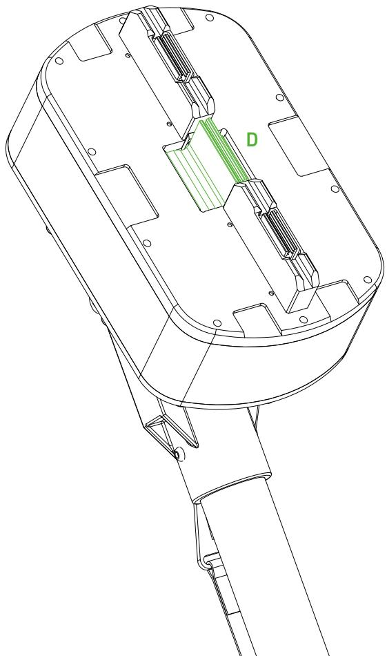
Position the first row of modules on the bar of the rails and use the GHOSTBUSTER to fix the middle clamp **D**.
