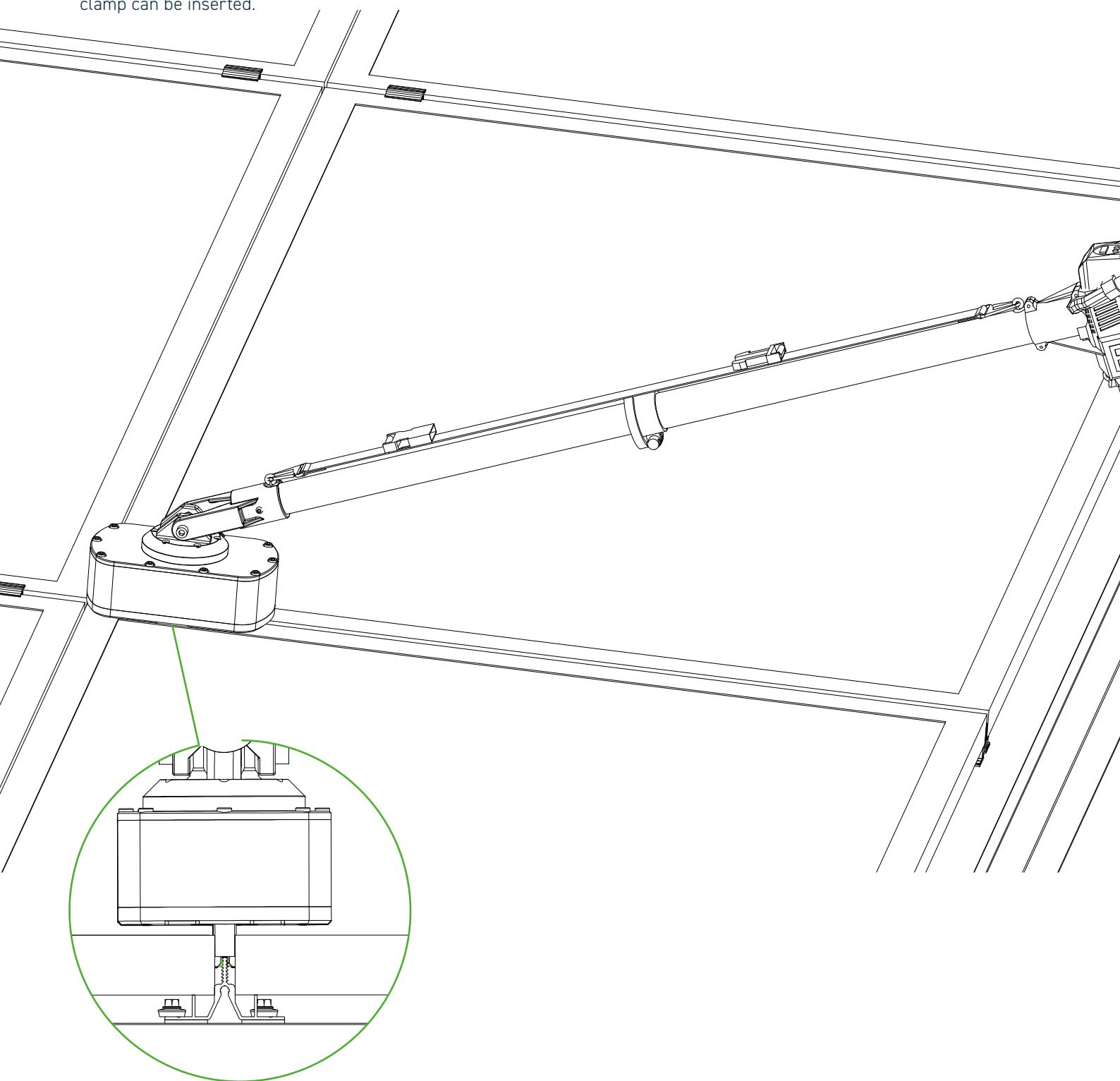
Position the first row of modules on the bar of the rails and use the GHOSTBUSTER to fix the middle clamp **D**.
