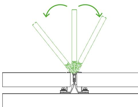
Move the dismantling tool back and forth in the direction of the wing to pry open the clamp.
